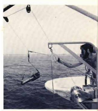
**7** A sound velocimeter can be lowered from the small hydrographic winch.
