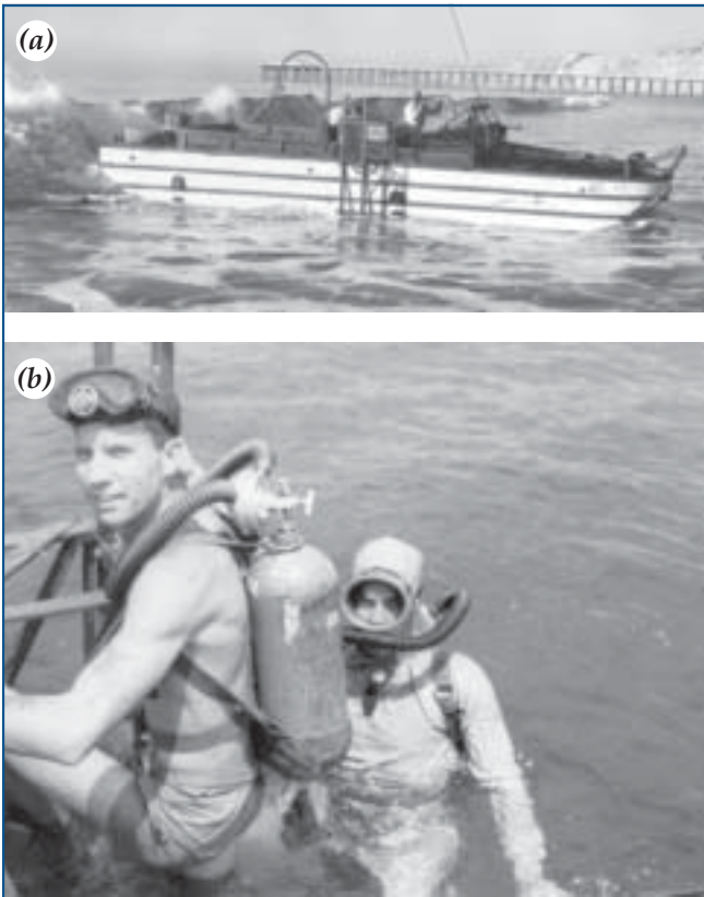
Figure 6. Surveying beach profiles off Scripps Pier (a) with a World War II amphibious DUKW provided by the U.S. Army Corps of Engineers and (b) aqualung divers, Earl Murray (left) and Walter Scott, returning to DUKW. Note the “dry” suit on Walter Scott (ca. 1950).
