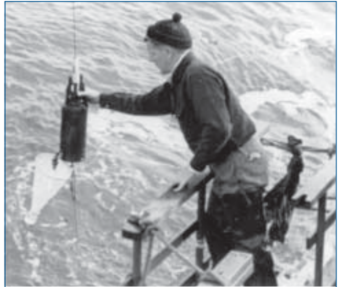
Figure 3. R.W. Fleming filtering a plankton sample captured with an Allen bottle.
