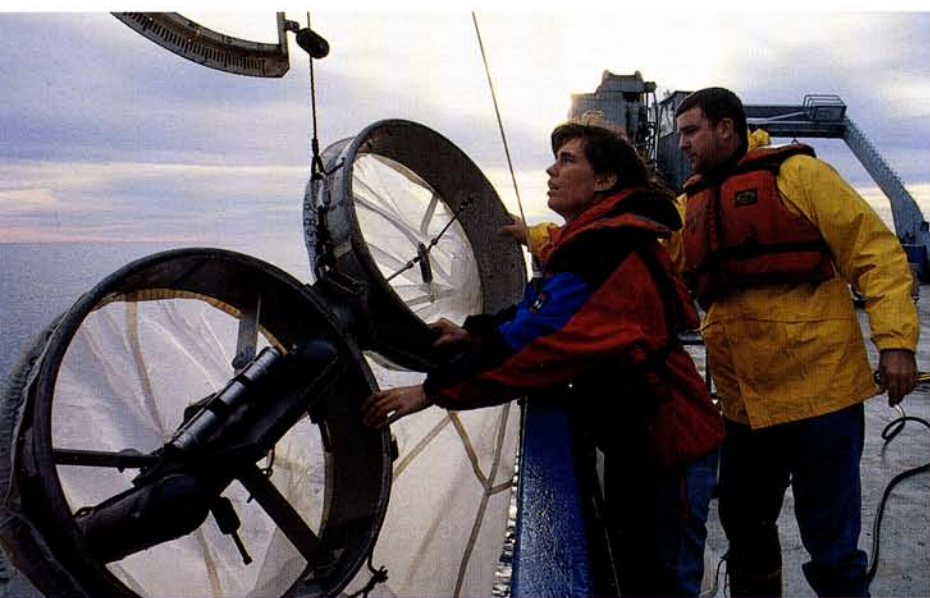
Amy Hayes, a fishery biologist with the SWFSC, and volunteer T. J. McCann prepare a bongo net for deployment. Created by McGowan and fellow Scripps researcher Daniel M. Brown in 1966, the net has become a standard device for zooplankton sampling.
