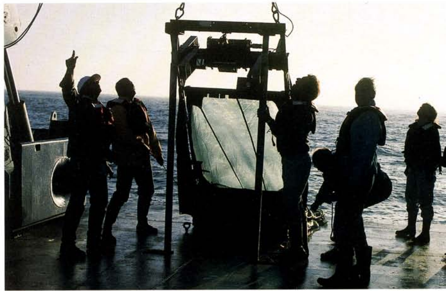
CalCOFI researchers conduct nine simultaneous hauls using this elaborate net system called a MOCNESS.
