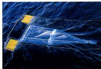
Above, The manta net (named for the animal it resembles) was developed at Scripps to collect fish eggs and larvae and other surface dwelling organisms as it skims the ocean. Below, A CTD rosette is deployed from R/V Roger Revelle.
