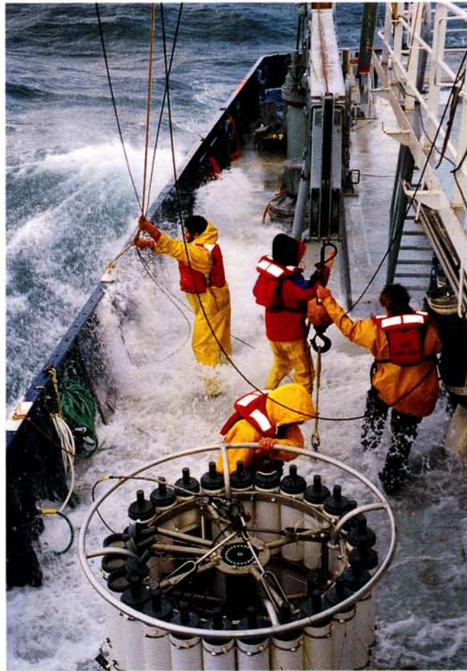
CalCOFI technicians use extra care deploying a CTD rosette in the wintertime waters of the California Current.
