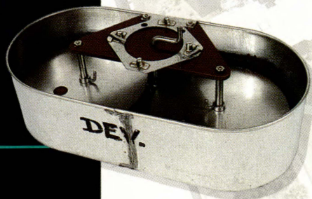
Film footage from Deep Tow's cameras was processed aboard ship using this developer can.
