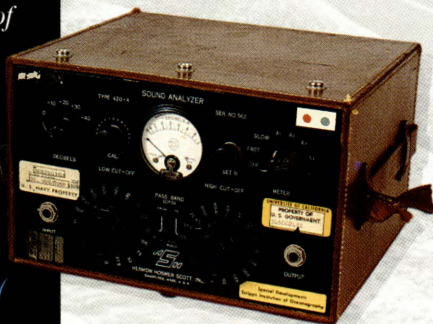
An early sound-spectrum analyzer, used in underwater acoustics research.
