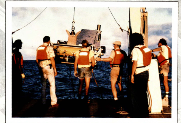
Precise scale model (above right) of Deep Tow , a remotely operated instrument package designed to be towed at depth by surface research vessels. Scientists aboard the Thomas Washington (right) used Deep Tow to study seafloor geology during the 1970 SEVEN-TOW expedition.
