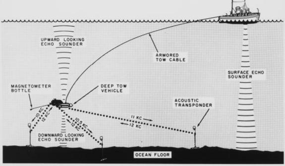
In this drawing the Deep Tow vehicle is making micro-topography and magnetic field studies of the sea floor while measuring its own depth with upward- and downward-looking echo sounders. It is shown using for precise navigation a sonar beacon network consisting of three acoustic transponders placed in a triangular pattern on the ocean bottom. During operations, the ship's echo sounder monitors the sea floor in advance of the Deep Tow vehicle.
