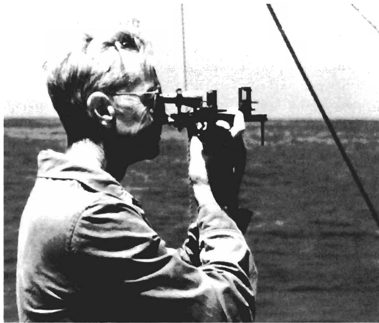
Shepard taking horizontal sextant angles for location of one of his many near-shore surveys, ca. 1975.
