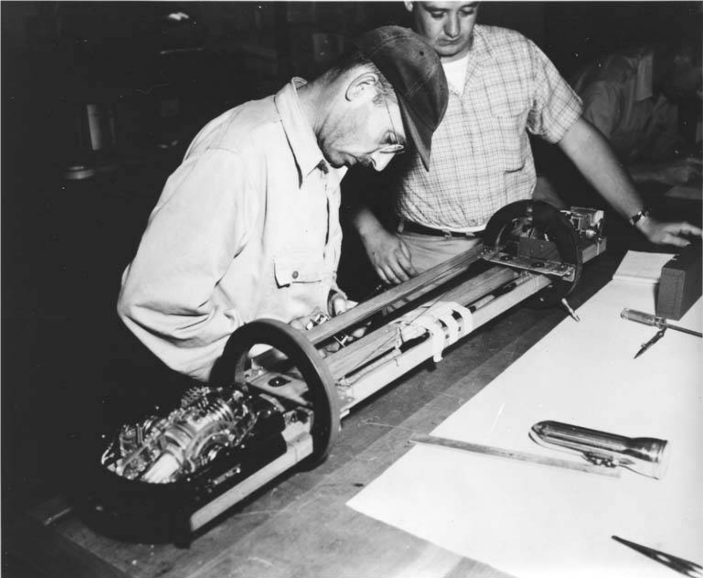
Arthur Datus Raff adjusting magnetometer sensor (out of towed "fish"). Aboard USC&GS vessel EXPLORER, 1960.
