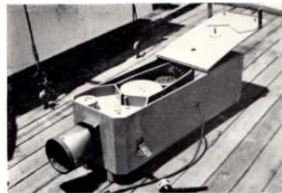
This machine - which I wanted to call a PTD for "plankton-temperature-depth" like STD - had by then come to be referred to as an LHPR (Longhurst-Hardy Plankton Recorder), a name which has stuck to today<sup>1</sup>: here is a modern LHPR, based on the design that we developed later at the NMFS Fishery-Oceanography Center at La Jolla -
