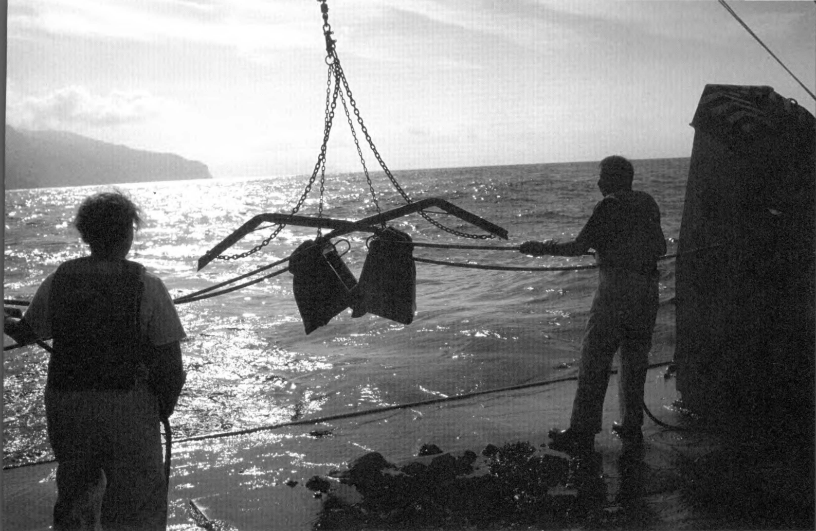
GRADUATE STUDENT KAREN CASCIOTTI AND RESEARCHER RICHARD COSSON USE A VAN VEEN GRAB IN THE SANTA BARBARA CHANNEL.
