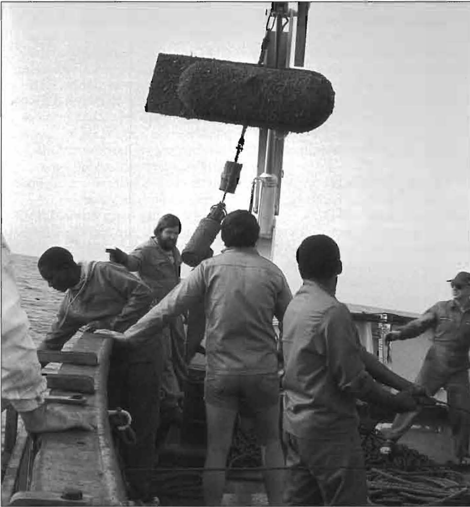
Deployment of a current-meter mooring from R/V Meiring Naude during the Agulhas Bank study.
