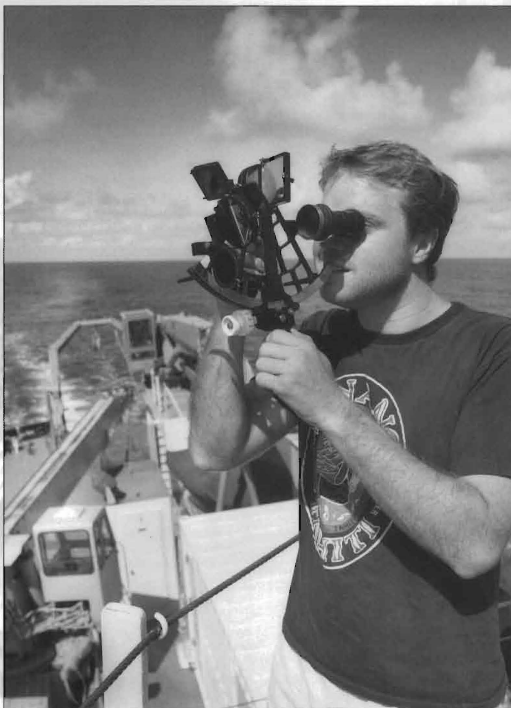
Wesley Hill uses a sextant to take a sunline aboard R/V Melville .
