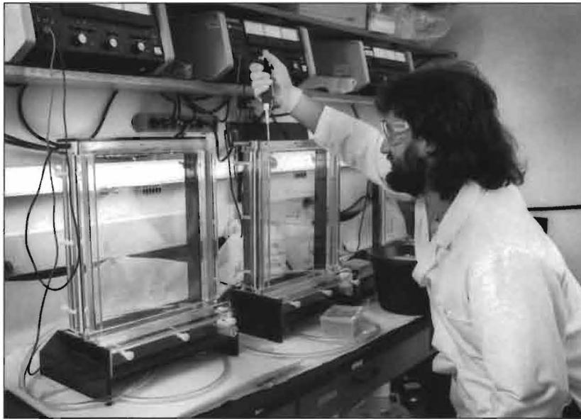
Scripps graduate student Richard G. LeDuc loads an electrophoresis rig to determine the sequence of DNA samples from dolphins.
