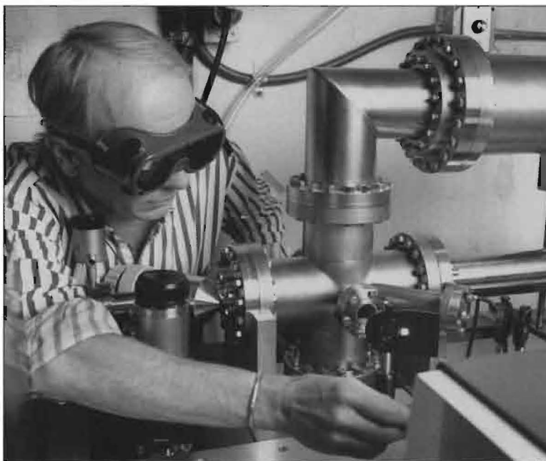
Dr. Bada uses a laser based detection system to measure polycyclic aromatic hydrocarbons.
