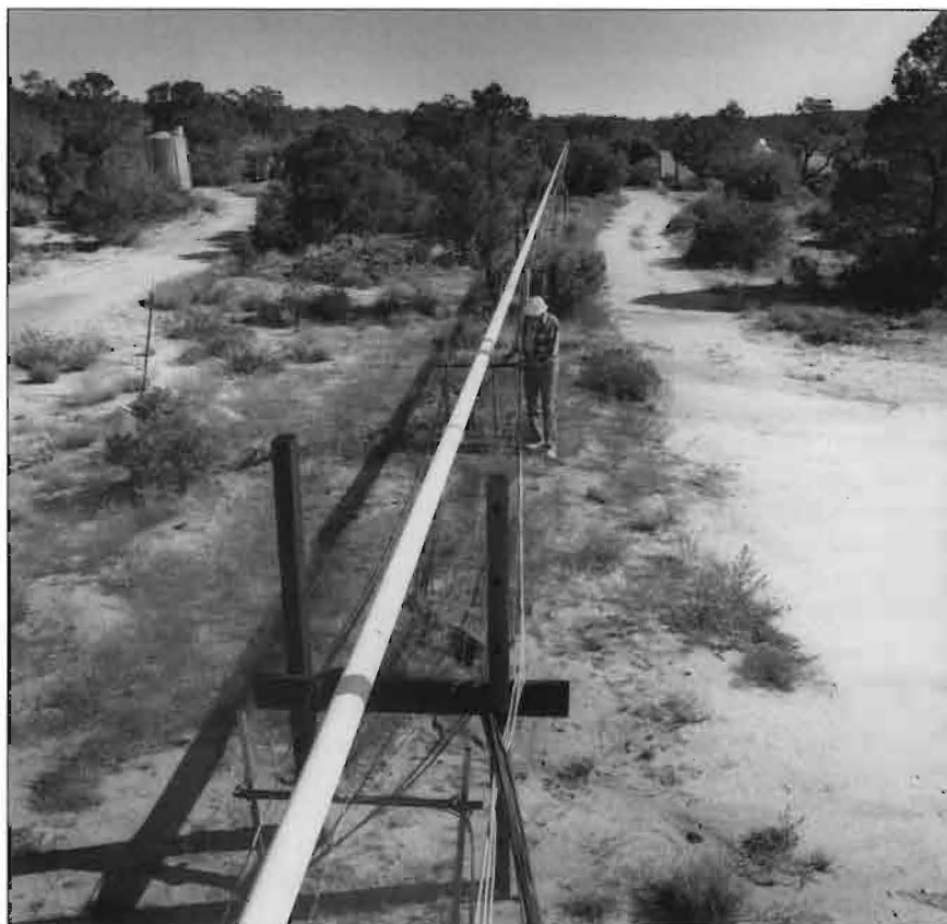
The 732-m long laser strainmeter at the Cecil and Ida Green Piñon Flat Observatory.
