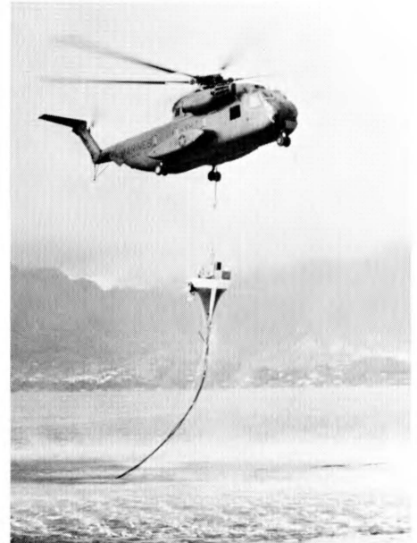
Unique launching of a model wave pump by a U.S. Marine helicopter from Kaneohe Bay, Hawaii, marked one of the Institute of Marine Resources' tests of a float attached to a 92-m-long pipe (portion of which is shown in photograph). Research indicated the pump, with its 5-cm-diameter pipe, magnified the pressure head more than 20 times. A by-product of operating this type of wave pump could be the fertilization of surface waters, provided the pipe is long enough to reach the entrained deep waters, which are rich in nutrients. Idea for such a wave-energy converter was that of John D. Isaacs. Dr. Gerald L. Wick and David Castel built and tested the converter under sponsorship of the State of Hawaii and its Natural Energy Laboratory.
