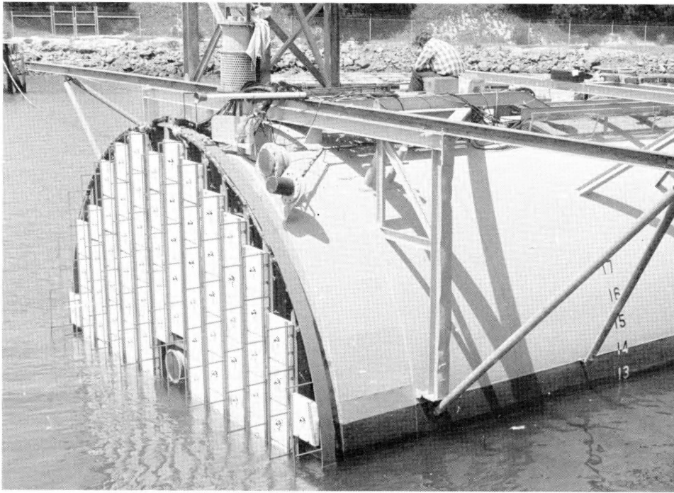
Mounted on bottom of R/P FLIP is Marine Physical Laboratory's acoustic scattering array (SCAR).
