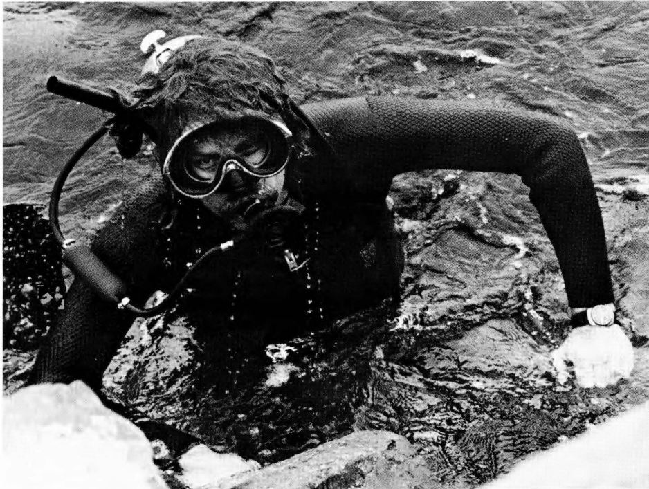
Graduate student James W. Stork emerges after a successful test dive wearing a breath heater and humidifier, a device developed by Stephen E. Suess, Foundation for Ocean Research, La Jolla, California, for SCUBA divers. Using about one percent hydrogen in the air tank and an oxidation catalyst, the device provides warm, moist air to the diver. It has been tested in the ocean and in laboratory tanks with encouraging results.
