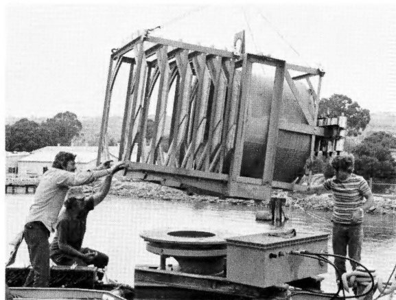
William R. Sessions, H. Wayne Wardlow, and Robert E. Bishop (from left), of Marine Physical Laboratory, mount doppler sonar on rotator base near bottom of R/P FLIP.
