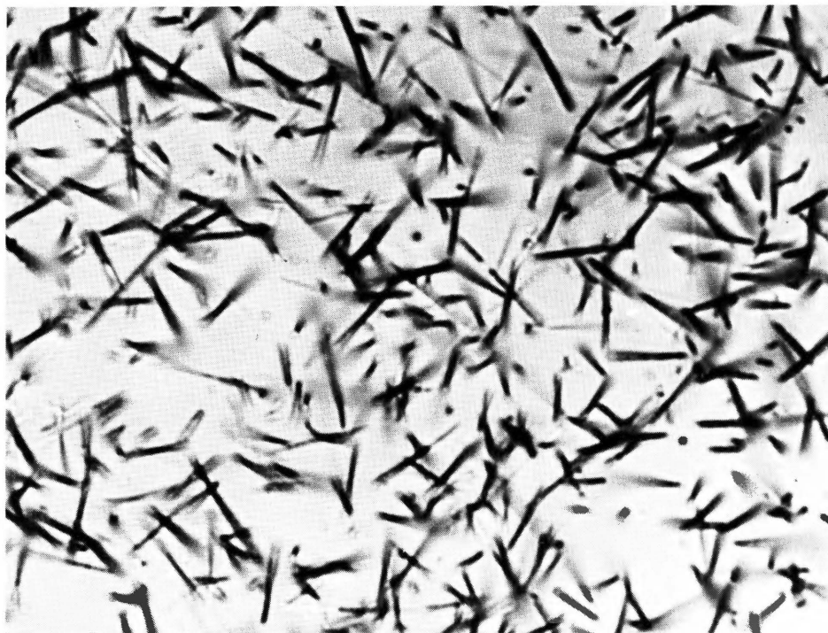
Among geochronological studies carried out during the year were those on fission-track dating techniques. Accompanying light micrograph shows fission tracks in a crystal of zircon. Each track is about ten micrometers long. Visibility of tracks has been enhanced by etching process that increases diameter of each track about 100 angstroms to a micrometer or more. Each track records spontaneous fission of an atom of uranium 238; as much as 1,000 parts of U-238 per million are found in zircon.
