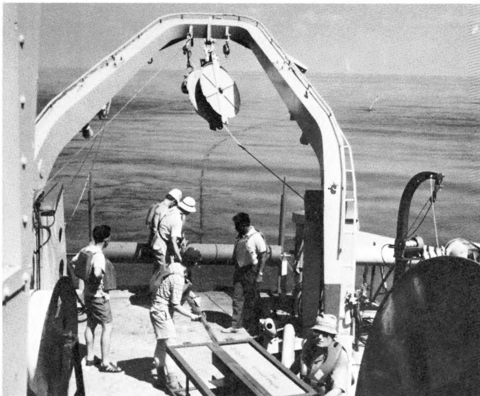
During geological and geophysical studies of the Andaman Sea, south of Burma, on Leg 11 of Indopac Expedition, technicians are shown deploying 2-km-long, seismic-reflection, hydrophone streamer from R/V Thomas Washington. The streamer, paying out from reel at lower right, passes through A-frame and into ocean. Surface tail buoy is barely visible to right of A-frame, about 100 m distant.
