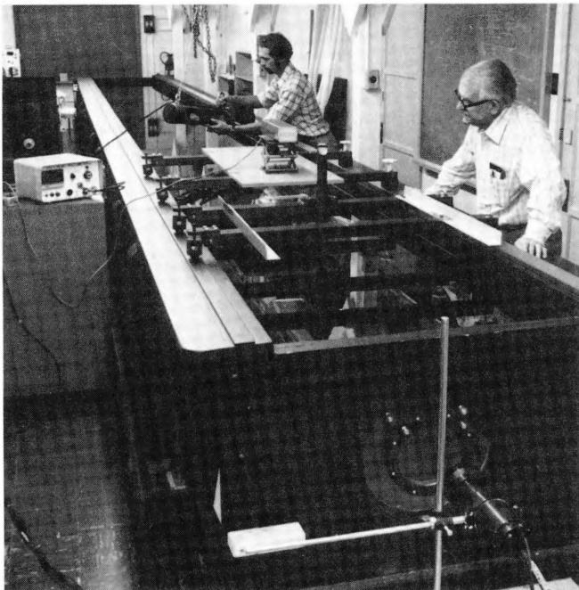
Using a new 13-m water tank installed at the Visibility Laboratory's Point Loma facility, investigators explore in detail the water properties affecting image propagation and perform controlled tests on new instruments for optical oceanography. Visibility Laboratory
