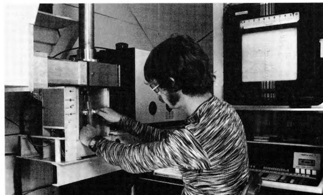
Newly developed computer-controlled flame spectrometer specialized for determining extremely small traces of alkalis in seawater at Mt. Soledad Laboratory. Multiple samples and standards are compared repeatedly under control and evaluation of digital system.
