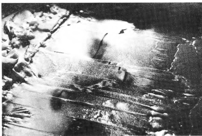
Upper figure is a map of Mid-Atlantic Ridge between Africa and South America which displays characteristic orthogonal pattern of ridges and transform faults. Lower figure is photograph taken from Oldenburg and Brune (1972), of an orthogonal pattern generated in a laboratory model by using candle wax. Upper photo: Copyright 1971 National Geographic Society; lower photo: Douglas W. Oldenburg.
