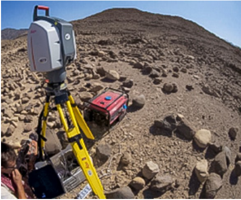
LiDAR laser scanner at Khirbat Faynan, where the expedition collected billions of geo-referenced data which to create 3D maps and computer models of the site.
