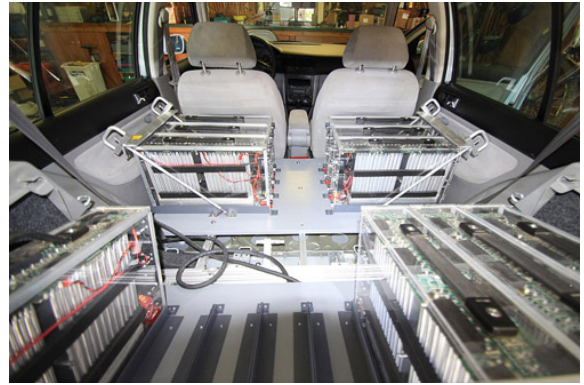
A snapshot of the inside of the Volkswagen Golf researchers outfitted with battery modules for their planned cross-country trip.
