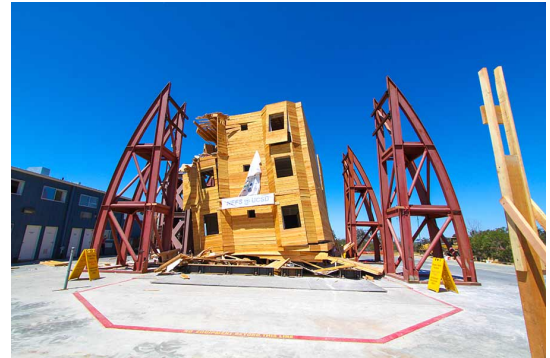
A wood frame building was tested to failure in 2013.
