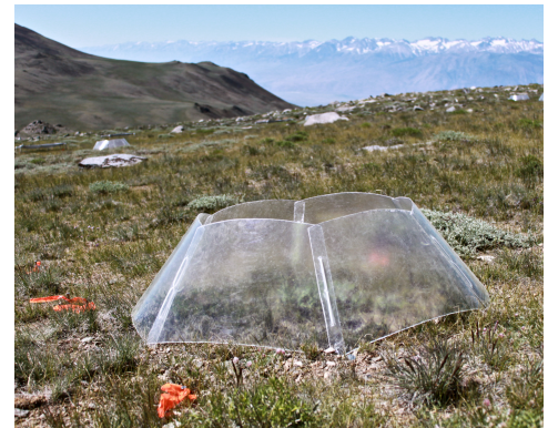
Open top warming chamber in the White Mountains of Ca Credit: Christopher Kopp
