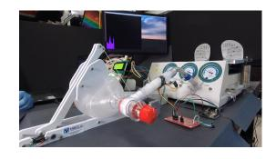
To measure pressure, the researchers developed an algorithm that deduces how much the bag was compressed based on how many turns the device's motor has made and calculates the volume of air sent into the patient's lungs as a result.
