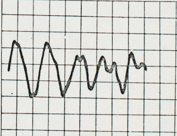
Oscilloscope tracings of amplifier output before filtering (1 volt per Abscissa Division and 50 milliseconds per Ordinate Division).
