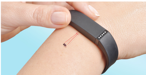
The wrist-worn wearable device is located above the sensor and transmits opioid measurements.
