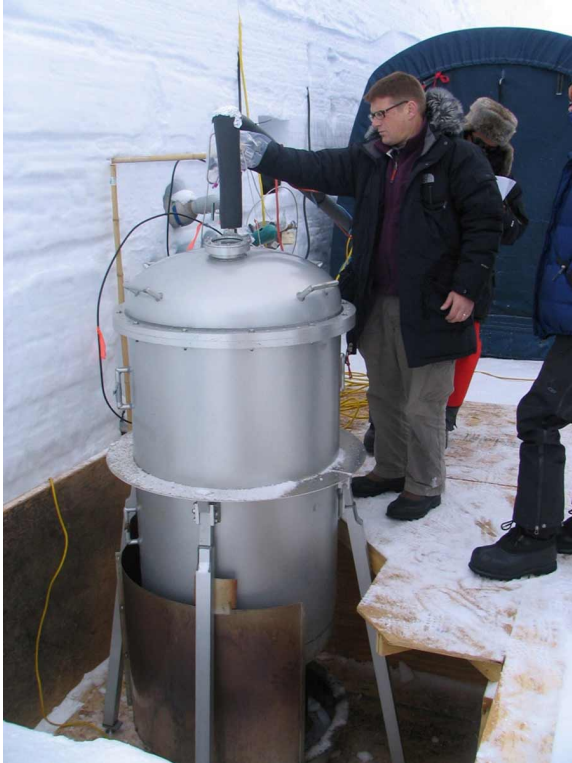
Scripps Institution of Oceanography geoscientist Jeff Severinghaus operates an instrument that separates air from the compacted snow that makes up Greenland's firn layer
