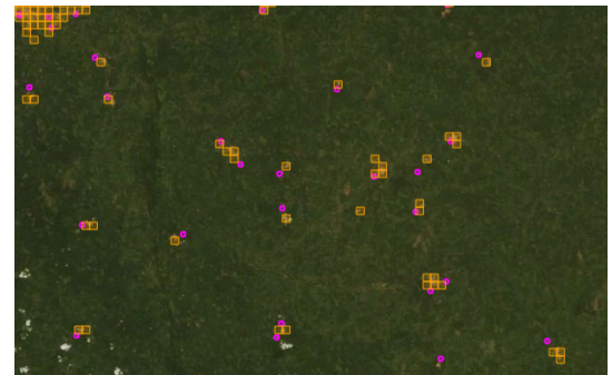
Validating the model's performance is accomplished by comparing its prediction of school locations with UNICEF's data. The orange squares represent tiles identified by the model as likely school locations, and the pink circles are actual schools from UNICEF's data. Courtesy of Mai Nguyen, SDSC
