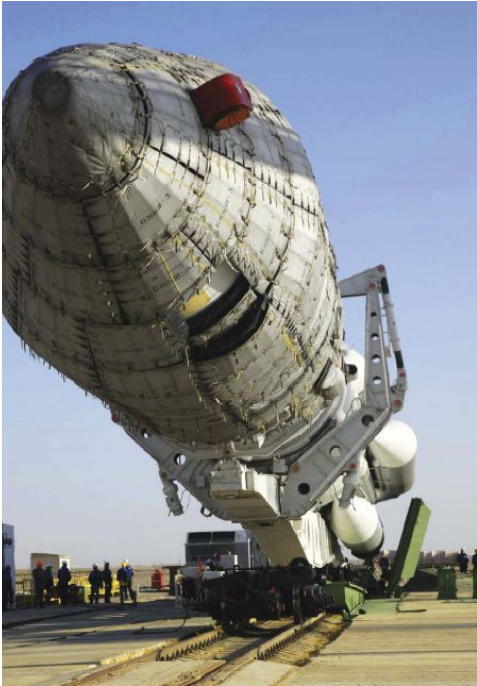
satellite, covered with grayish panels, sits atop the railcar transporter. It will be tilted up to vertical launch pad, and the panels removed.
