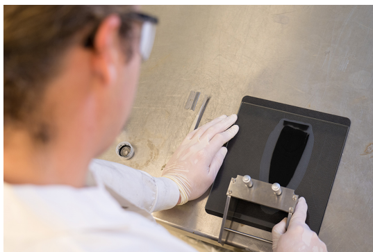
To make the new separator, a slurry of polymer gel is casted onto a glass slide, followed by a layer of carbon nanotubes.
