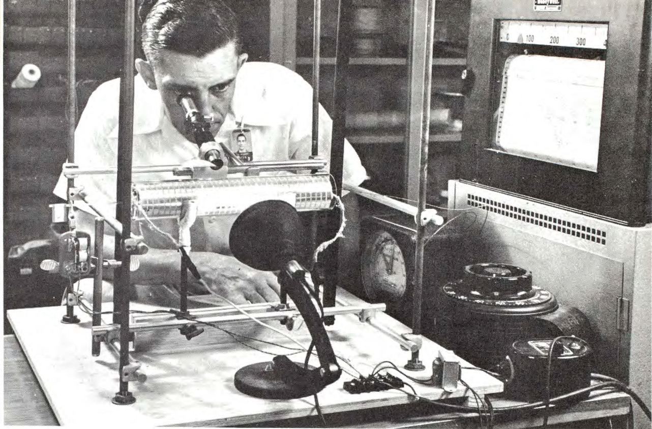
High-temperature solubility studies. The spiral object is a heater, and the investigator observes the dissolution of crystals contained in a small tube within the heater.
