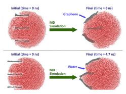
One layer of graphene is so thin that it takes a million layers to make it one millimeter thick. A simulation done using SDSC's Comet supercomputer shows a crosssectional view of seven graphene flakes in a water droplet, and that the multi-layered graphene eventually merges together. Credit: Solanky et al. Computational Materials Science, 162(2019)
