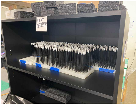
Trays QI mechanical engineer Alex Grant designed and manufactured to hold the swabs in easy-to-count rows to streamline the process throughout the production line.
