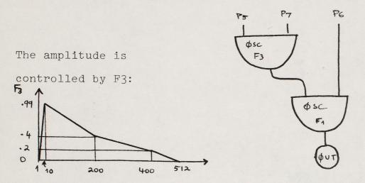
For a duration smaller than about .2s, this function will give a sharp attack; the decay consists of 3 linear portions: the 2 first approximate an exponential shape, the 3rd tries to imitate the effect of a damper.
