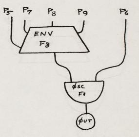
exponential attack time of 10 milliseconds which corresponds to a very sharp attack, and an exponential decay time varying between .5s and 2s. The tone quality reminds of a plucked string instrument.
