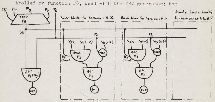
maximum amplitude of this component is determined by P5, and has to be smaller than 512. The output of the ENV generator is input-output block B3. B3 is used as amplitude input of the
