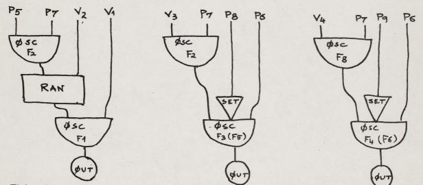
This instrument gives a sound which is the sum of a frequency band and of an inharmonic spectrum. This sound decays exponentially.
