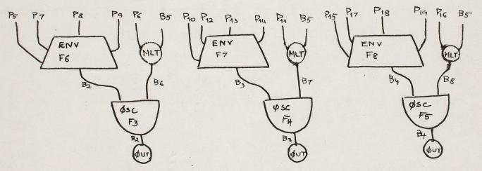
One of these oscillators generates the fundamental of maximum frequency 160Hz (F3 is a sine wave.). The amplitude is controlled
