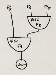
Note: here the rate at which the frequency controlling functions are scanned is determined by P7 (converted by P(7)=F/P(7)): it is divorced from the duration of the note; in effect these functions are scanned several times for one note length.
