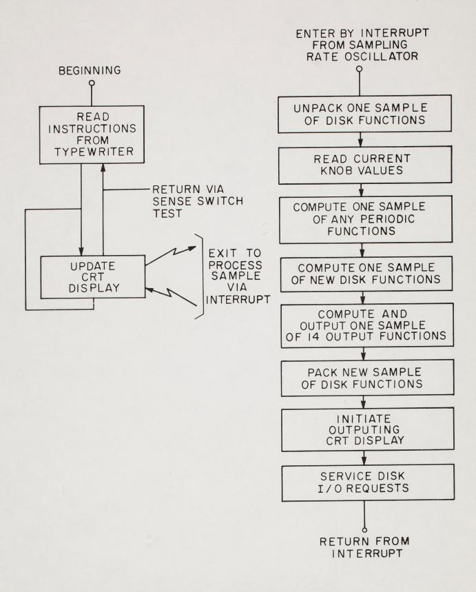
FIG. 4-BLOCK DIAGRAM OF GROOVE PROGRAM
