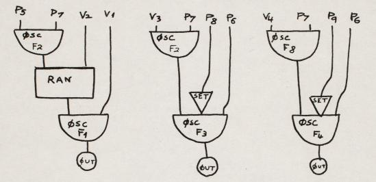
This instrument gives a sound which is the sum of a frequency band, of a sine wave and of an inharmonic spectrum.
