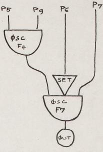
The first section compares linear and exponential decay. Linear decay is controlled by function F4:
