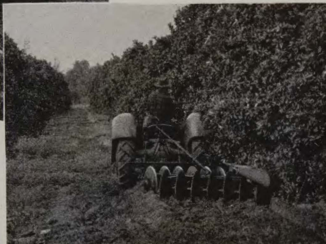
A new lift type 5' 3" Towner Disc Harrow used in an offset operation.
