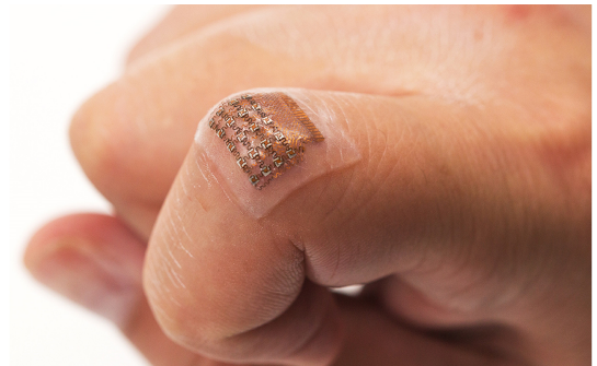
Wearable ultrasound patch tracks blood pressure in a deep artery or vein. Images courtesy of Chonghe Wang/Nature Biomedical Engineering
