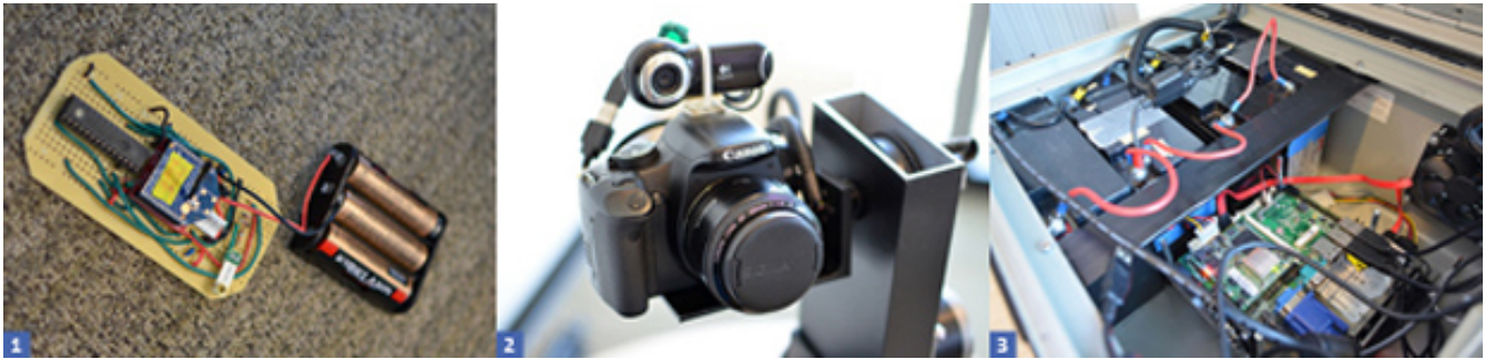
Components of the camera trap system include 1) wireless, piezoelectric vibration sensors, 2) camera and turret, and 3) inner workings, including Intel Atom processor and stepper motors.
