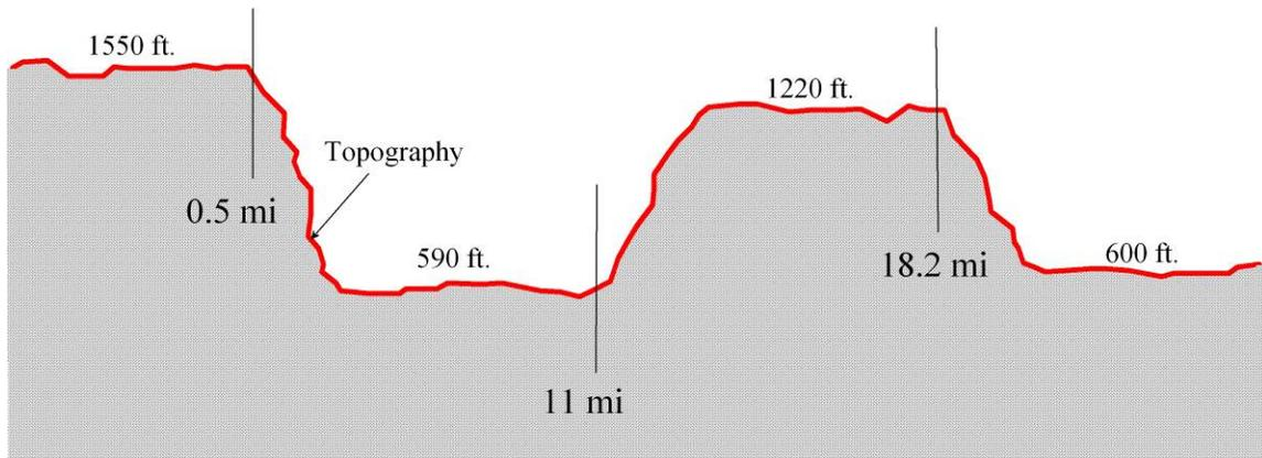
**Figure 3:** An example of NCALM flight planning. Topographic profiles of the site (along planned flight lines) are used to schedule maneuvers, such as climbs, descents, changes in heading, to ensure maximum data uniformity.
