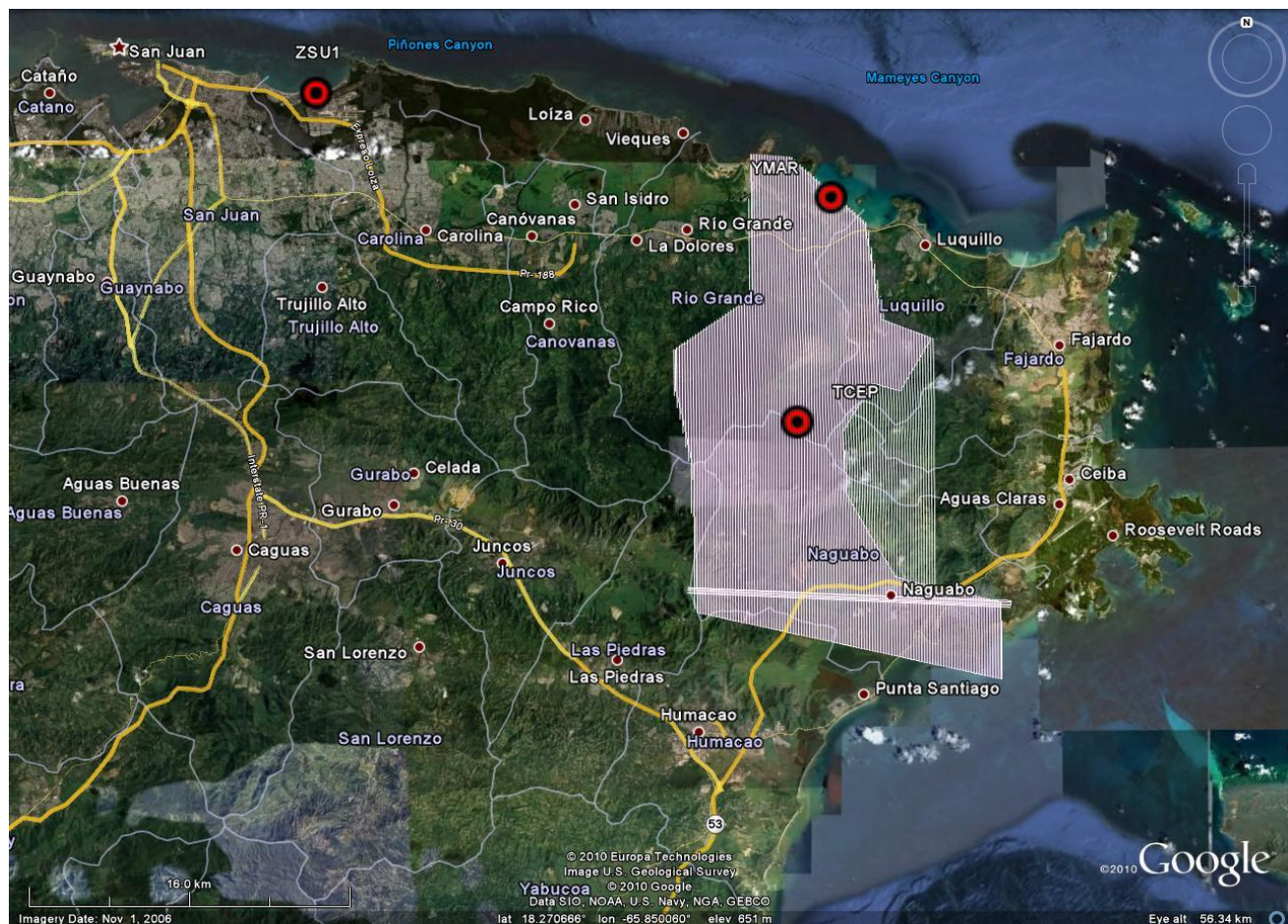
Figure 14. Area of interest (AOI), flight lines and GPS stations for the Luquillo, Puerto Rico CZO sub-project.
