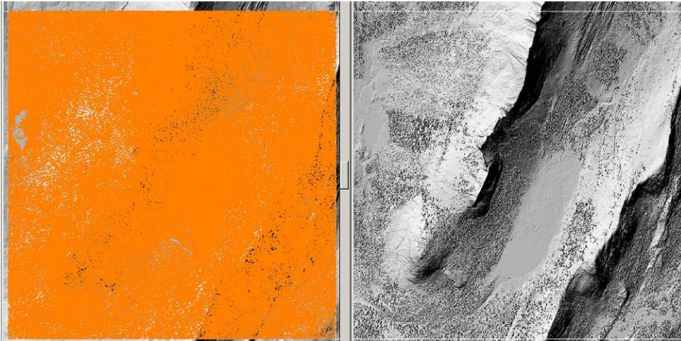
**Figure 6b:** Yosemite Block 25 detail view. The main ridge is far better preserved after semi-manual classification and filter tuning.
