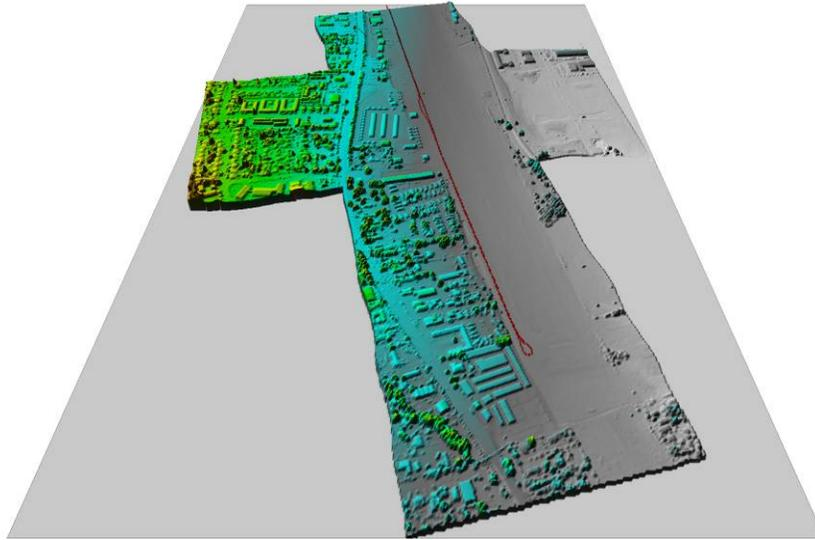
**Figure 2:** Orthogonal ALSM calibration swaths taken over an airport used during a deployment. Kinematic GPS ground points (shown in red) are used to calibrate the system in the field.
