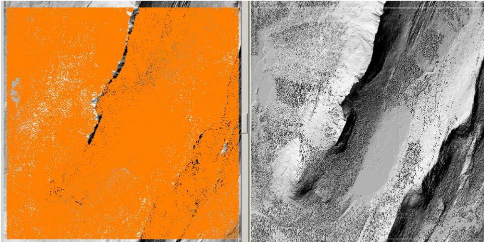
**Figure 6a:** Yosemite Block 25 detail view. Initial filtering omitted points on the tops of very sharp ridges (orange = points classified as ground)
