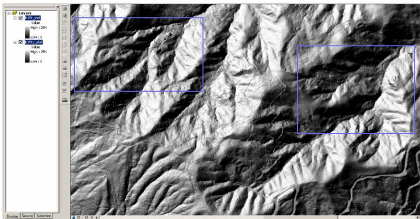
**Figure 5b:** Marshall Block 1 detail view after initial filtering. Note loss of detail caused by low density of ground points and the subsequent interpolation (kriging) artifacts.
