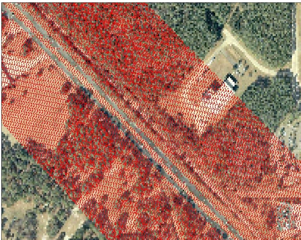
**Figure 4. Laser shots from raw file posted on a section of a city street in another area of the survey.**
