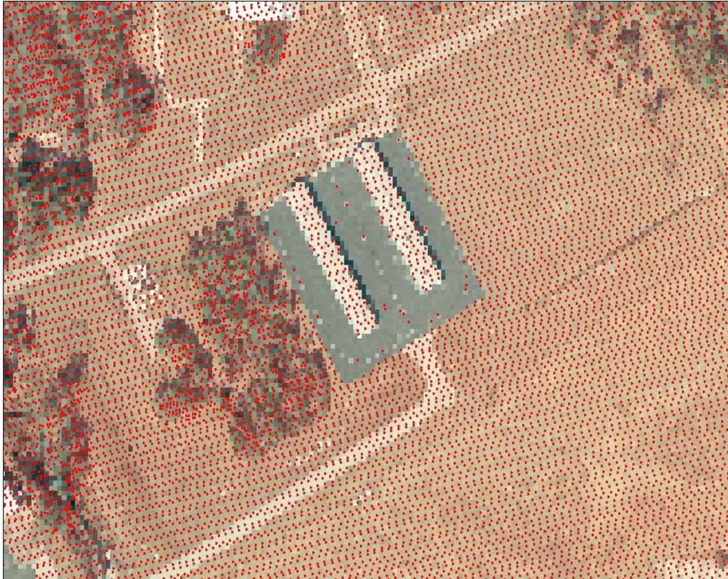
**Figure 3. Laser shots from raw file plotted over an area of dark asphalt surrounding hangers at the airport.**
