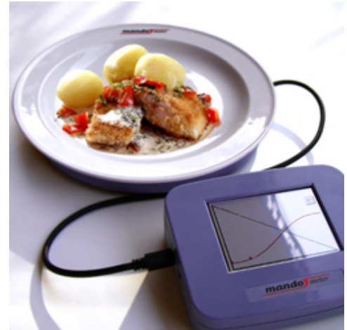
The Mandometer’s small scale and monitoring system provides feedback on eating behavior, training patients how to normalize their eating pattern and eat less without feeling hungry. Credit: Jenny Nilstam, The Mando Group.
