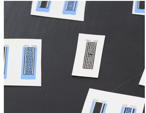
Printed biofuel cells designed to convert wastewater, urine and sewage into energy are being developed for military applications. Joshua Windmiller, a postdoctoral researcher in the Nano and Nanobioelectronics Laboratory of Professor Joseph V.lasser, Department of NanoEngineering, Jacobs School of Engineering, is one of four researchers from Southern California who receive a von Liebig Center fellowship to pursue the commercialization of renewable energy sources.
