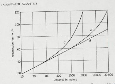
Fig. 15.1. Curves showing dependence of transmission loss on distance and frequency. Curve A at 1 kc/sec. Curve B at 10 kc/sec. Curve C at 50 kc/sec.
