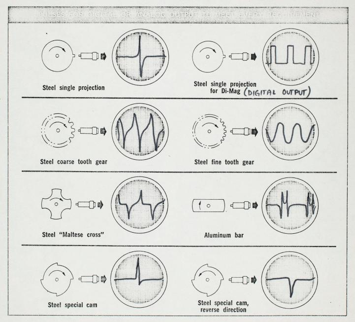
Generally speaking, gears are the most frequently used actuating mass. As shown above, actuators of varying sizes and shapes produce different waveforms. Fine tooth gears generate a near sine wave output, while coarse tooth gears produce a sharply peaked pulse. However, the same results can be obtained by utilizing wheel spokes, a vibrating surface, a moving bar, crank, or even a steel screwhead mounted on a moving surface.
