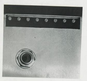
DETAIL OF CONTROL INPUT AND 15 TURN TRIMPOTS FOR ADJUSTING FREQUENCY.
