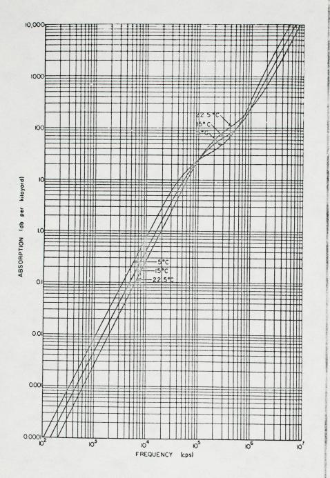
Figure 3. Absorption of sound in the ocean as a function of frequency, with temperature as a parameter.
