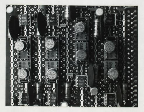
DETAIL OF HIDDEN SIDE OF CIRCUIT BOARD, Relays, IC's, and external components.
