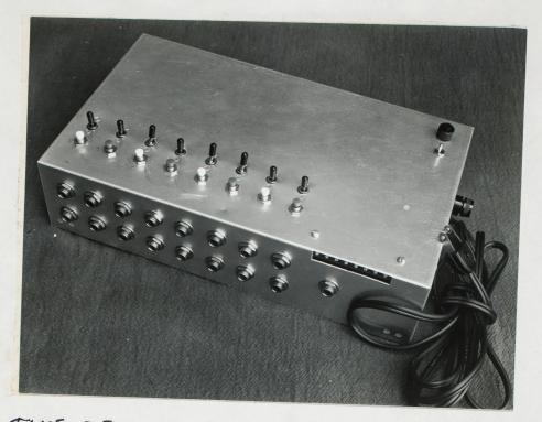
TONE DECODING SWITCHING SYSTEM: VIEW OF TOP & FRONT PANELS.
