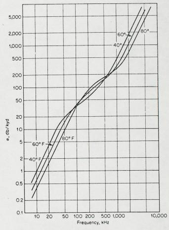
Fig. 5.3. Absorption coefficient in seawater of salinity 35 ppt as a function of frequency at three temperatures.
