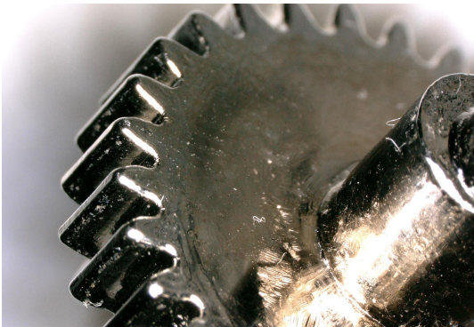
Components of wear resistant gears made out of bulk metallic glass. Image courtesy of NASA/JPL-Caltech.
