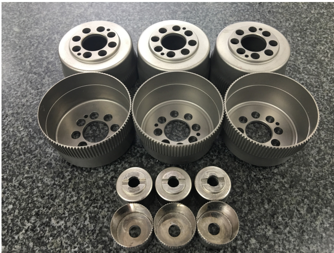
Components of wear resistant gears made out of bulk metallic glass. Image courtesy of NASA/JPL-Caltech.
