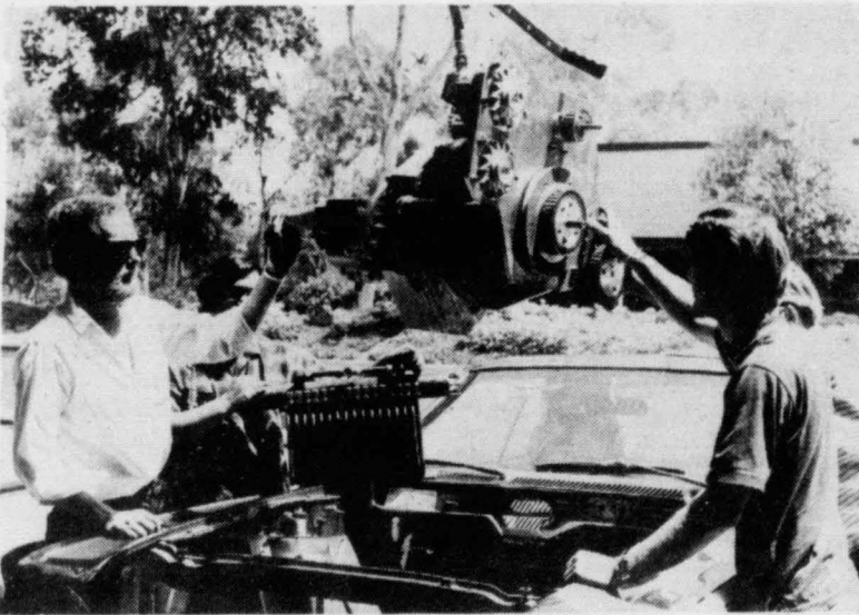
UCSD grad student lowering newly developed propane engine into university
