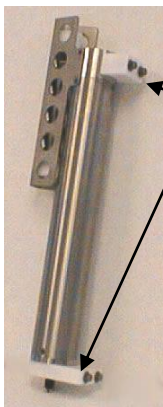
Mounting clamp and guide – loosen hardware to separate clamp/guide halves and mount on mooring cable
