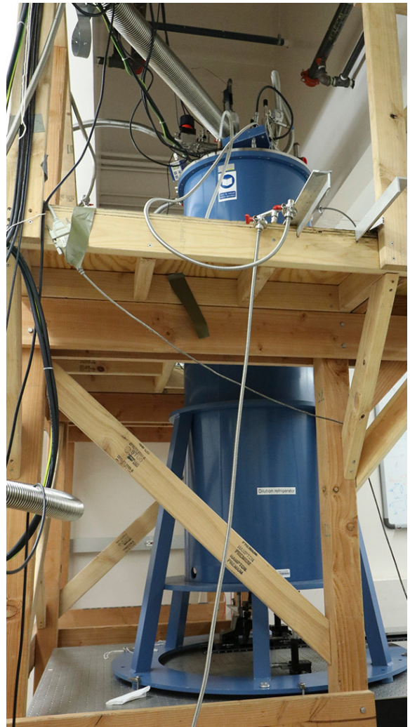
Optical dilution refrigerator for low-temperature experiments at UC San Diego. Photo by Michelle Fredricks
