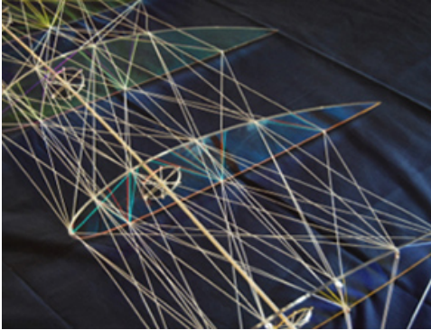
Robert Skelton displays an airplane wing made of balsa wood and tensioned string - an example of tensegrity, which also allows it to be malleable, flexible and adaptable.
