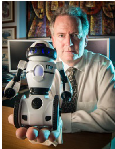
MAE Prof. Tom Bewley holds the MiP toy robot with a self-balancing control system developed in Bewley's UCSD lab.
