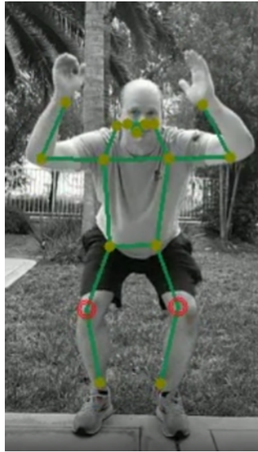
Figure 10: Video Feedback to users indicating when and which joint the incorrectness was observed
