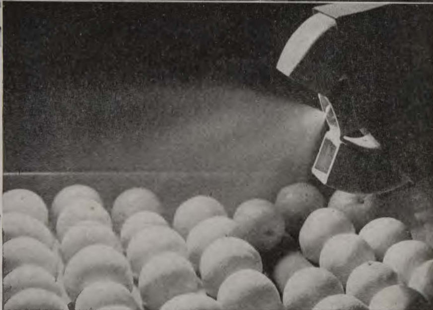
Here are oranges under the spray nozzle of the special machine developed to apply the FLAVORSEAL protective film.
