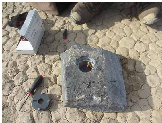
A rock with the cavity that held the GPS instrument package and its battery pack. This rock, MAIA, traveled 162.4 m in several move events during the time the pond existed on the Racetrack, starting with a 64.1 m move on December 20 2013. credited to Richard Norris
