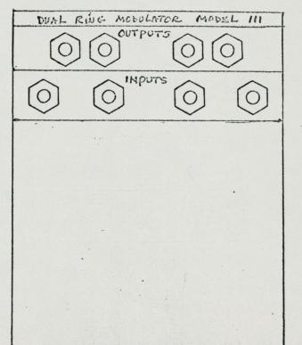
RING MODULATOR REQUIRES 2 SEPARATE ADDIO SIGNALS. THE FUNDAMENTALS ARE SUPPRESSED AND THE SUMS AND DIFFERENCES (COMBINATION TONES) ARE AMPLIFIED.
