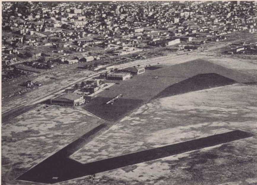
Lindbergh Field is equipped with a 3000-foot runway, and three 2,500-foot runways. At the extreme right may be seen the "birthplace" of the "Spirit of St. Louis" now occupied by the Solar Aircraft Company, manufacturers of exhaust collector manifolds for practically all of the leading aircraft manufacturers in the country.
