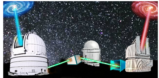
Schematic of the 2018 “Cosmic Bell” experiment at the Roque de Los Muchachos Observatory in the Canary Islands, where two large telescopes observed the fluctuating color of light from distant quasars (red and blue galaxies). The green beams indicate polarization-entangled photons sent through the open air between stations separated by about one kilometer. Image by Andrew S. Friedman and Dominik Rauch
