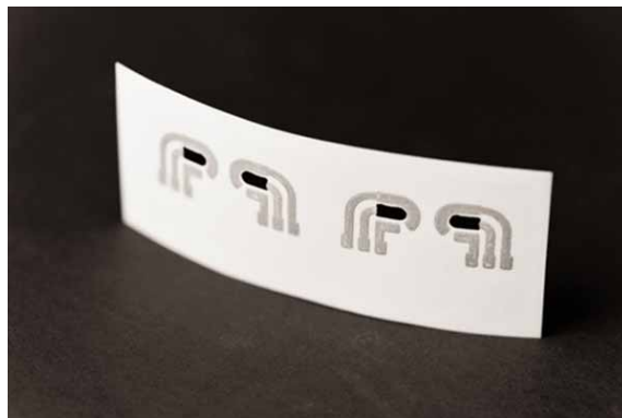
The device consists of carefully patterned electrodes printed on temporary tattoo paper.
