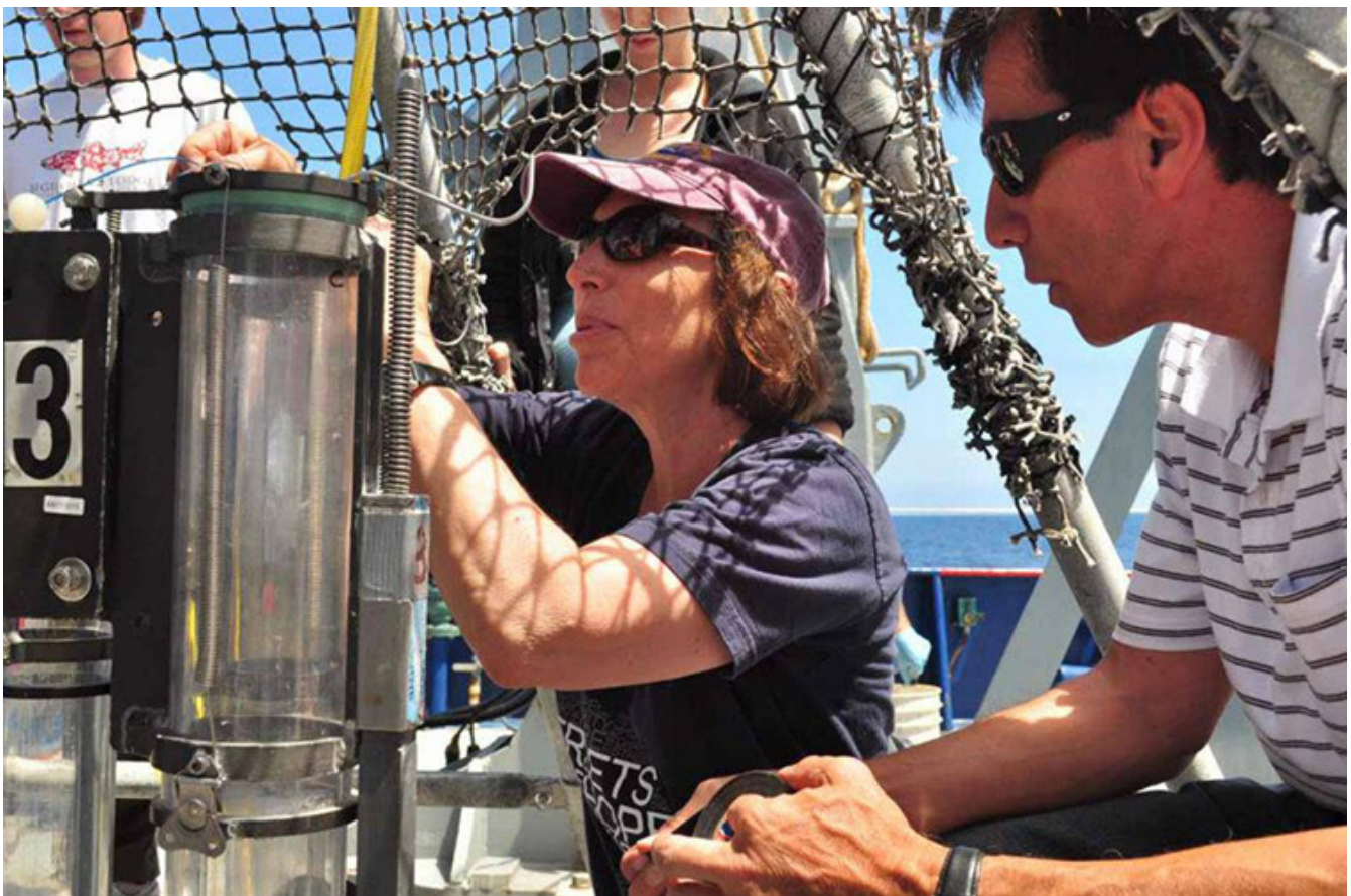
Scripps scientists Lisa Levin and Carlos Neira preparing a sediment coring instrument for deployment on the seafloor.
